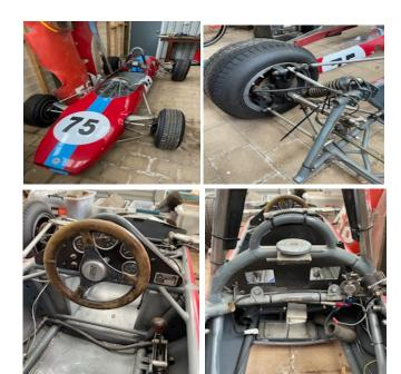
Now ... Current condition of the car is best described as "as last raced". The 1300cc Alfa Romeo twin cam and Colotti-Francis five speed have been removed from the car. General condition of the car is good, albeit it will need some refurbishment and recommissioning. Chassis tubes appear very sound and, importantly, the top radiator rail to the engine shows the tube is in very good shape with minimal surface crusting. The original Cooper magnesium wheels are in good shape. Included with the
