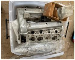
Original 998cc cam cover with Alfa plate denoting build, block underneath.
